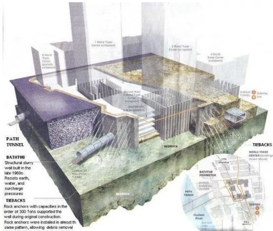
Exhibit 1: World Trade Center Bathtub and Original Conditions (adapted from NY Times 9/18/01)
